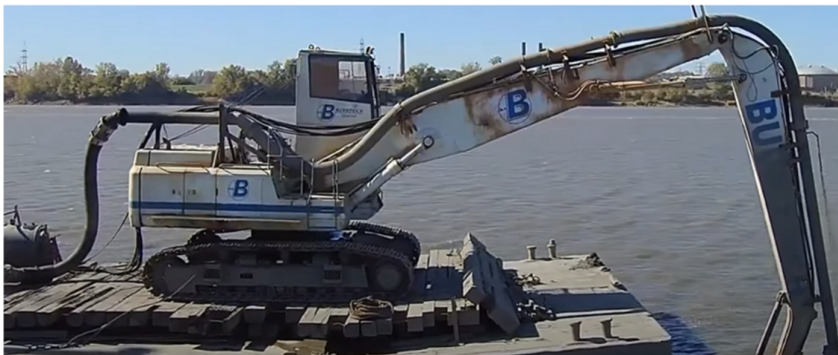
Pictures: Pontoon operated excavator (left) and cutter head attachment
