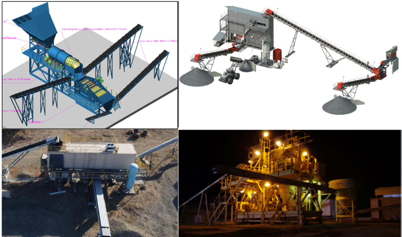
Pictures: 150 tph Scrubbing and screening module acquired in 2023 (top left) Tomra Com 300 XRT module acquired in 2023 (top right) existing Tomra Com 1200 XRT module (bottom left) and the existing Bateman 15 tph DMS (bottom right)
