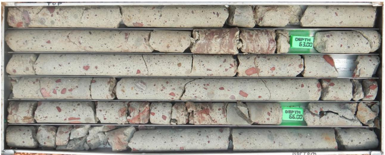
Figure 3: Kimberlite core intersected in E4
