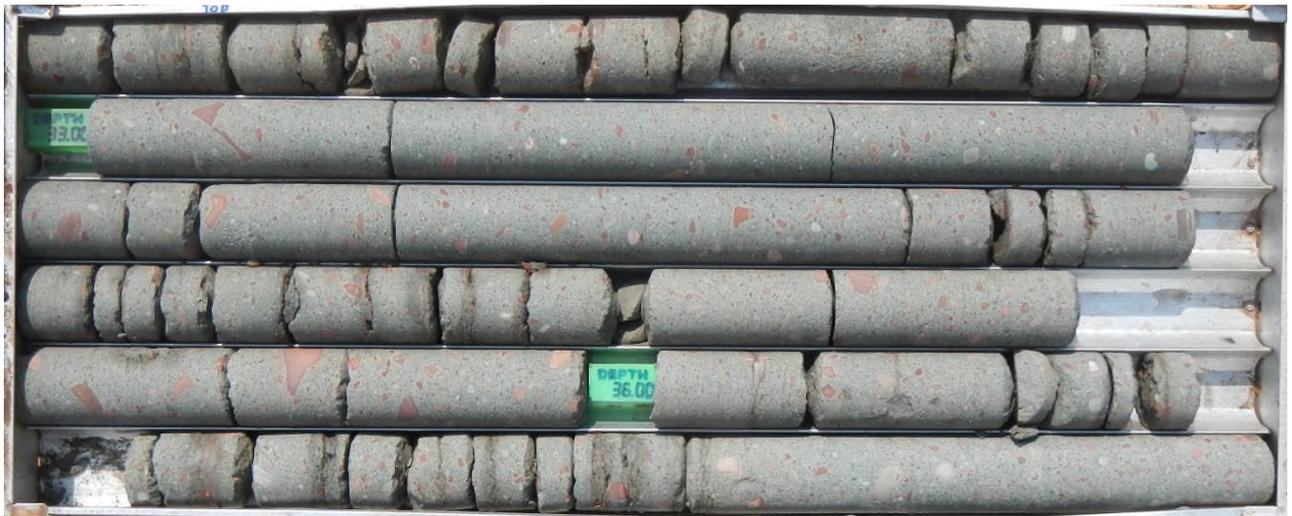
Figure 2: Kimberlite core intersected in G510
