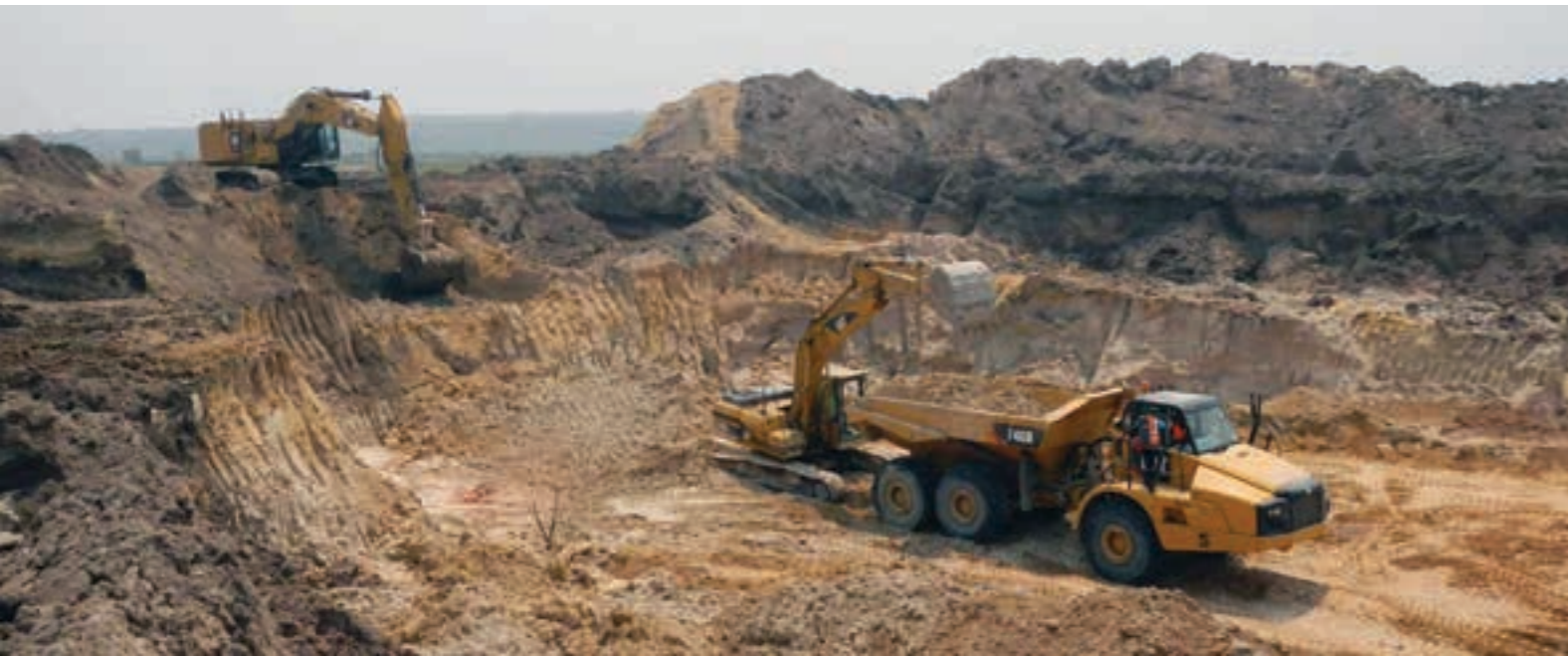
Alluvial mining at Lulo in Angola. Mining at the site is currently running at a rate of 20 000 bank cubic metres per month.
